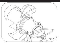
• Fit the visor, lower visor and the canopy as shown (Fig.5); Secure in place with M5x10 bolts.
